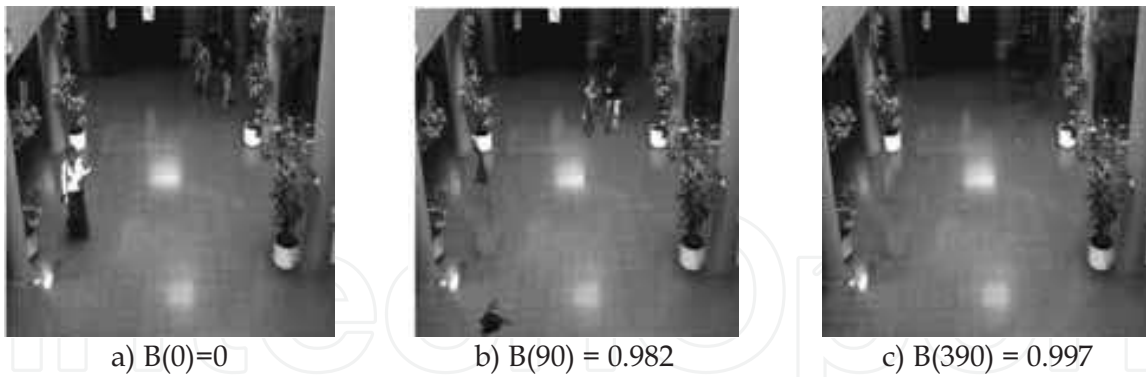
Fig. 2. Background evolution, first figure correspond to background model in F (1). Figure (b) corresponds to the background model updated until F (90). Figure (c) corresponds to the background model in F (390).
