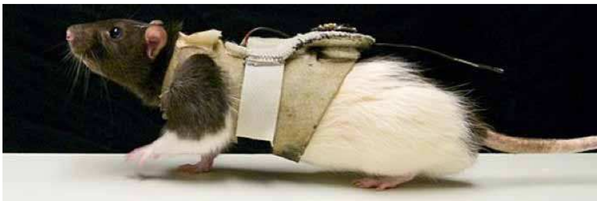
Fig. 1. An example of a laboratory rat wearing a mica2dot sensor node on a removable harness
