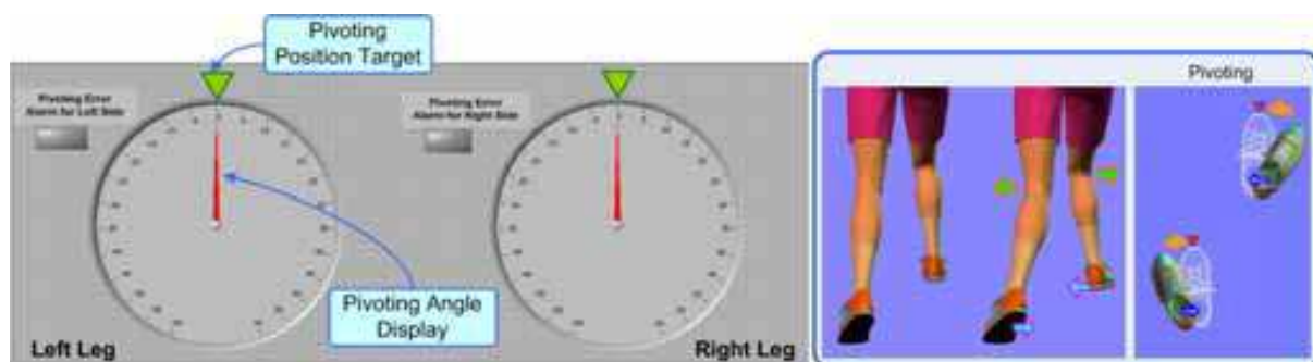
Fig. 5. Real-time feedback of the footplate position is used to update a virtual reality display of the feet, which is used to help the subject achieve proper foot positioning
