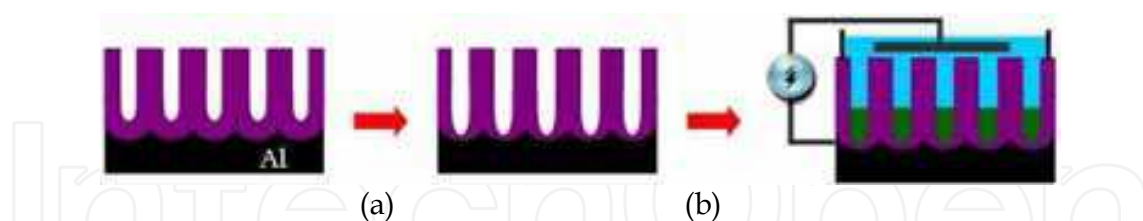
Fig. 6. Fabrication of MNWs via on-substrate AAO/Al template: a) barrier layer thinning, and b) AC electro-deposition.
