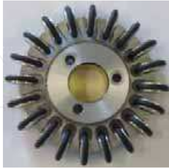
Fig. 1. 5DPO omni-directional wheel
