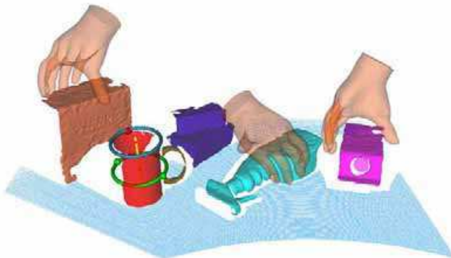
Fig. 1. Detected grasping points and hand poses. The green points display the grasping points for rotationally symmetric objects. The red points show an alternative grasp along the top rim. The illustrated hand poses show a possible grasp for the remaining graspable objects 1 .
