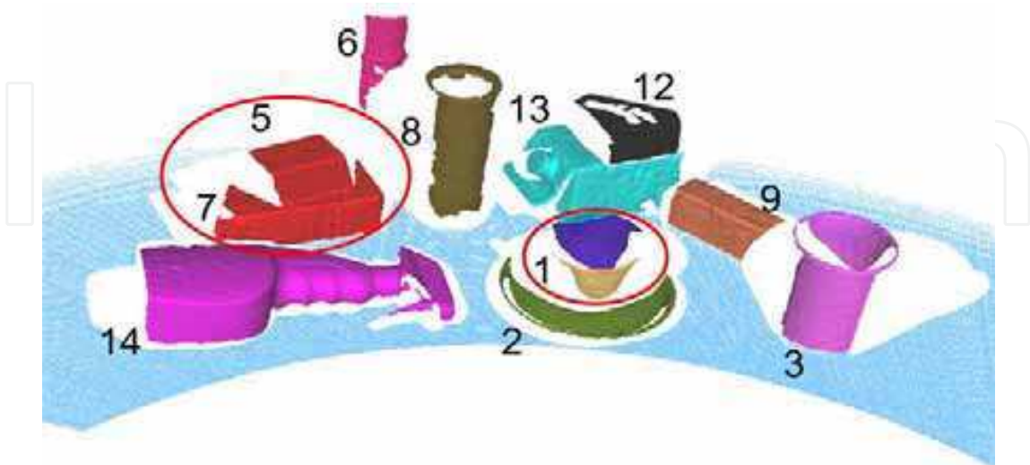
Fig. 5. Results after the first segmentation step. Object no. 1 is cut into two parts and objects no. 5 and 7 are overlapping. The not perfectly segmented objects are red encircled
