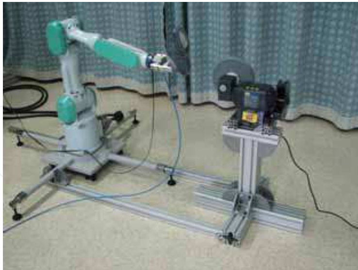
Fig. 5. Experimental cell for shoe bottom roughing
