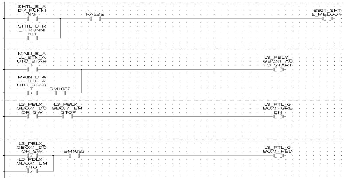
Fig. 1. The PLC code in the form of Ladder diagram
