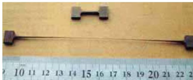
Fig. 4. Tensile specimen made of Zr_{41.25}Ti_{13.75}Cu_{12.5}Ni_{10}Be_{22.5} alloy following superplastic forming in the supercooled liquid region (Wang et al., 2005).
