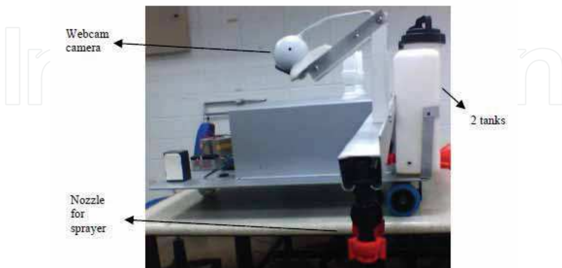
Fig. 3. The sprayer structure of the automated weeding strategy
