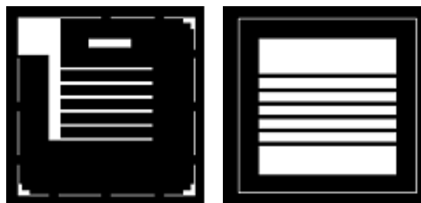
Fig. 10. Masks of device fabrication by MIMIC process.
