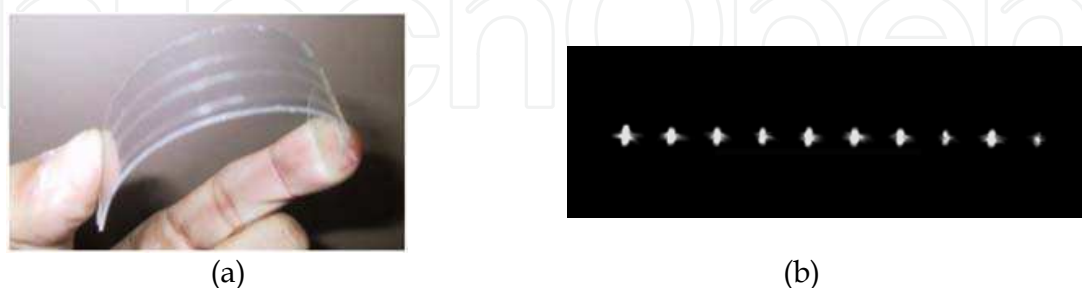
Fig. 8. a) Flexible ribbon array waveguide on co-polyester substrate and b) resulting output mode spots emerging from waveguide array device.
