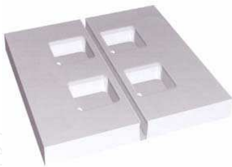
Fig. 21. Simulated 3D resist profiles for the layout in Fig.20 after exposure with 100 keV He + ion beam
