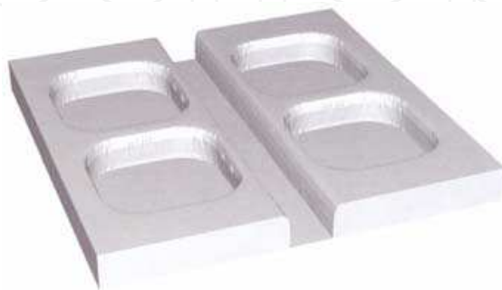
Fig. 20. Simulated 3D resist profiles for a layout consisting one 30 \text{ nm} wide line and four 800 \times 800 \text{ nm}^2 squares at 50 \text{ keV e} -beam
