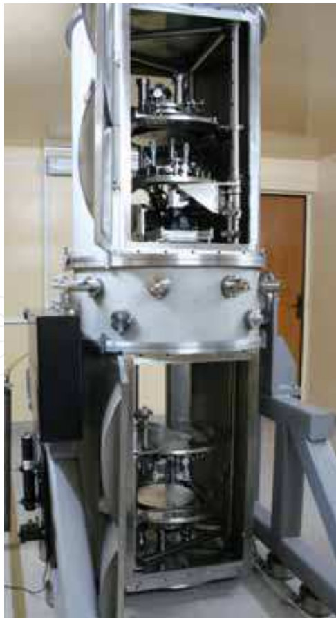
Fig. 16. Photograph of the vertical vacuum interferometer.
