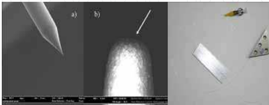
Fig. 11. Photographs of the fiber based source taken with scanning electron microscope (marked as a) and b)) and the source with on optical connector.
