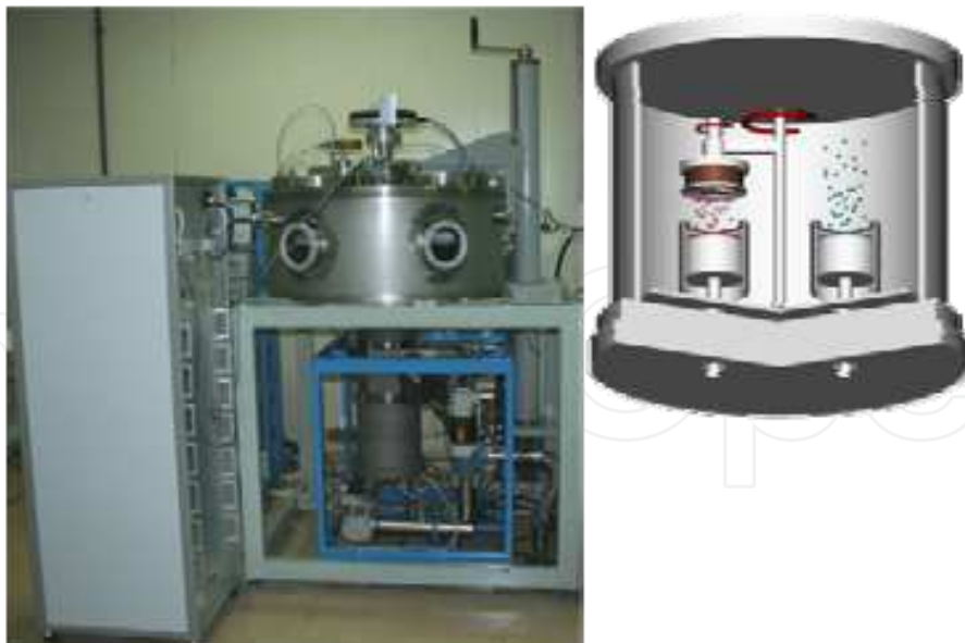
Fig. 24. Photograph of a technological facility and scheme of surface shape correction by means of multilayer film deposition through masks.
