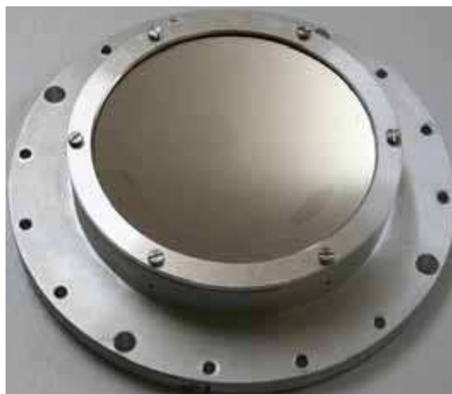
Fig. 33. Photograph of the multilayer spherical mirror for 13.5 nm wavelength in the frame. Diameter of the working aperture is 130 mm.
