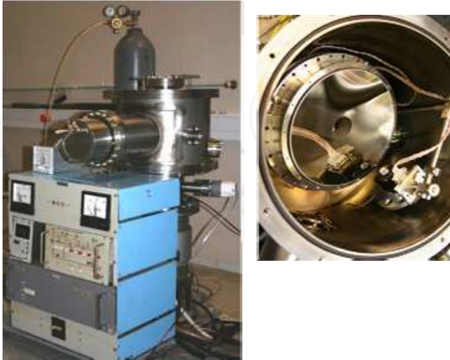
Fig. 26. Photographs of installation for substrates surface shape correction by ion-beam etching.
