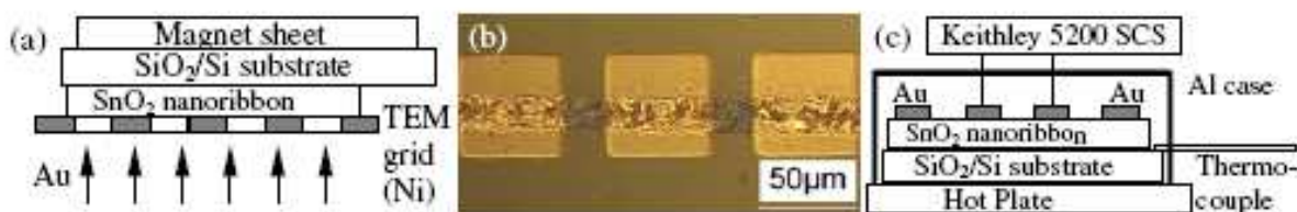
Fig. 2. Deposition of Au contacts along a single SnO 2 ribbon using TEM grids as masks: (a) schematics, (b) optical micrograph of resulting sample, (c), schematics of the testing system.
