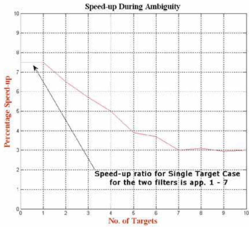
Fig. 3. Kalman & Alpha-Beta Filter Speed-Up Comparison
