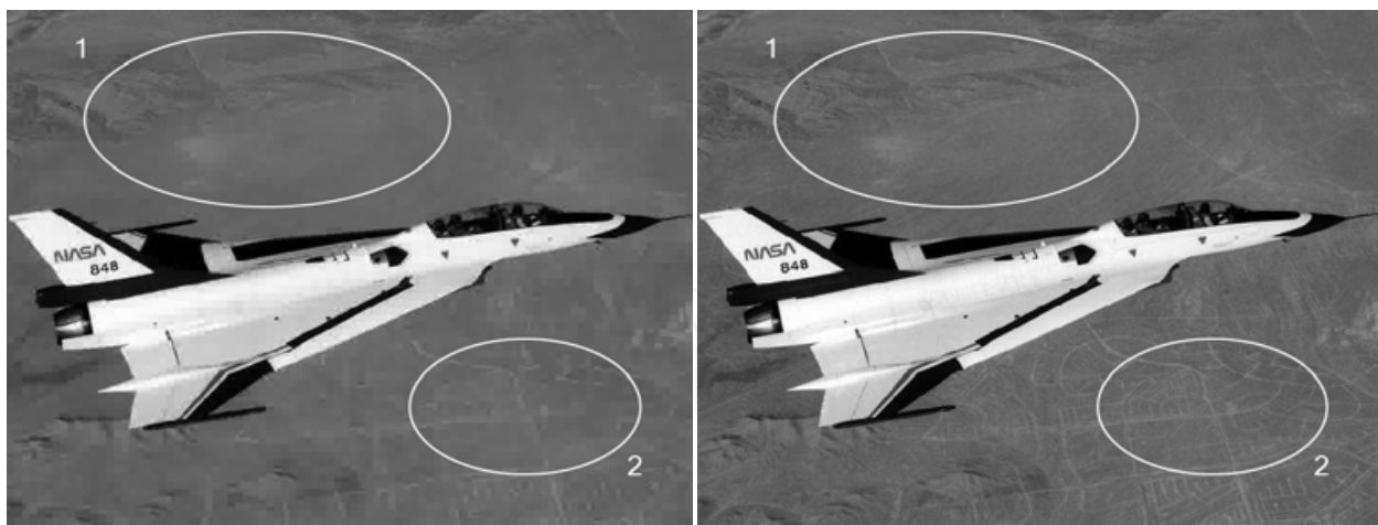
Fig. 1. 13. Image compressed with MPEG-2 (compression ratio is 75) Fig. 1. 14. Wavelet based image compression (compression ratio is 45)
