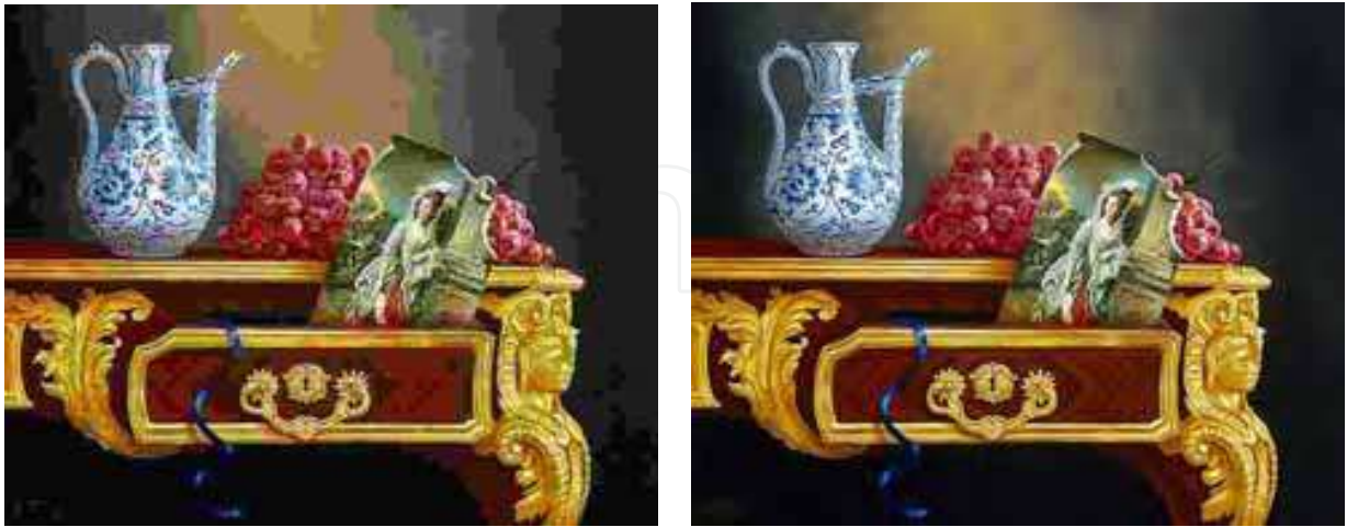
Fig. 1. 22. Comparative quality of images on the basis of JPEG and JPEG-2000 at Cr=100
