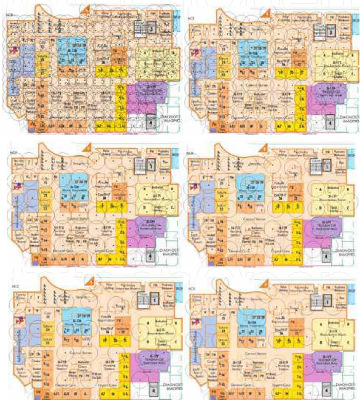
Fig. 5. RFID reader configurations (top left to bottom right: reader spacing at 100, 150, 200, 250, 300, 350 pixels).
