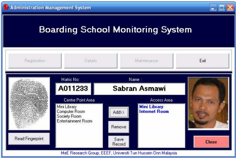
Fig. 13. Access Registration of Facility at Zone 1 Accessing Zone 1 acquire extra identification system. In this application, the identification used user’s fingerprint. Therefore, each user needs to register one of their fingerprints into the system. The fingerprint is registered into BoS system by clicking the Register Fingerprint button. By doing so, the fingerprint reader reads the fingerprint and sends it to the system before displaying it to the user and save it into the database. The overall flow of registration process is shown in Figure 14.
