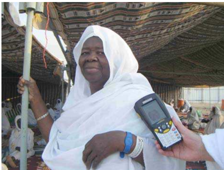
Fig. 15. Information of a pilgrim is displayed on the handheld reader as it is brought close to the tag.
