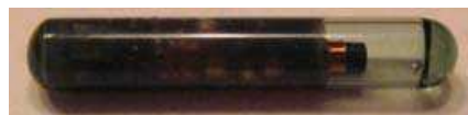
Fig. 4. The smallest glass transponder, 12 millimetres long and 2.12 millimetres in diameter, used for the tests.
