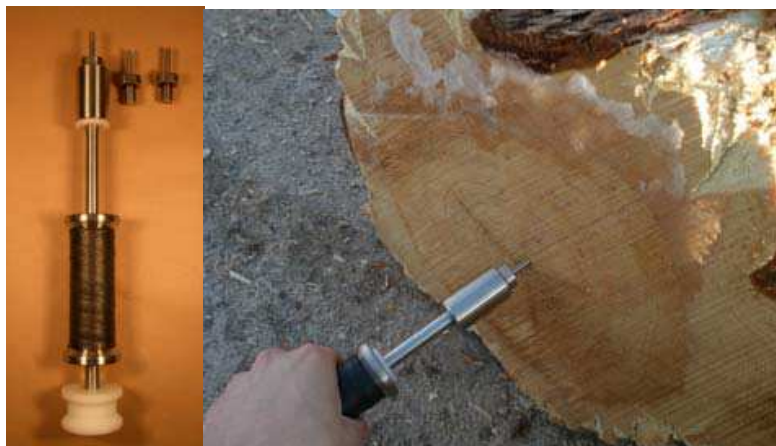
Fig. 8. Left: Tool for manual application of transponders. Right: Manual application of transponder to log.
