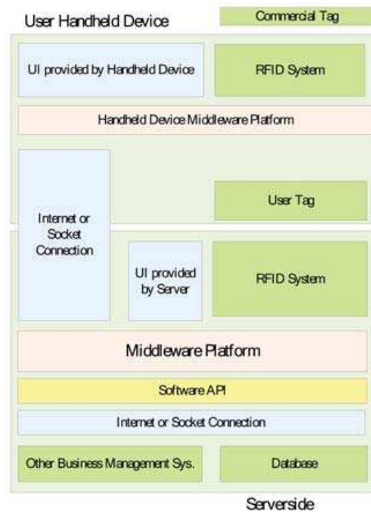
Fig. 5. The framework of service application with RFID system.
