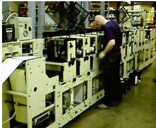
Fig. 2. Image of a multi-station flexographic printer. Printed trace thickness can be adjusted by letting two or more stations print with identical printing plates.
