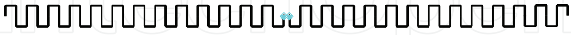
Fig. 7. Meander-line antenna on a single substrate ( \epsilon_1 = 2.2 , d_1 = 1.58 mm, G = 4.6 dBi, W = 263.8 mm and H = 11 mm).
