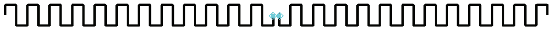
Fig. 9. Meander-line antenna on a single substrate ( \epsilon_1 = 2.2 , d_1 = 1.58 mm, \epsilon_2 = 2.2 , d_2 = 1.58 mm, G = 4.81 dBi, W = 243.8 mm and H = 11 mm).
