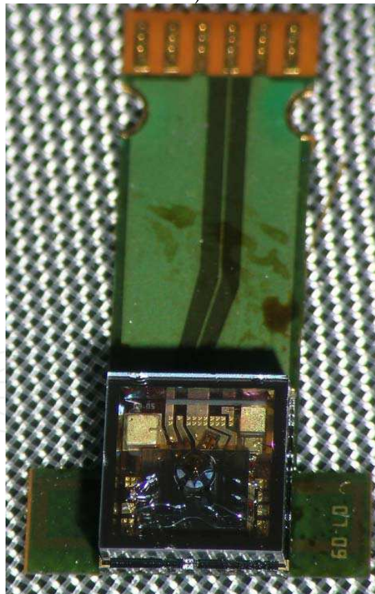
Fig. 13. Assembly of the MEMS device. a) Flowchart of the assembly process. b) Fully assembled system comprising flexprint, MEMS, microlens, electronic components, laser diode and glass lid.
