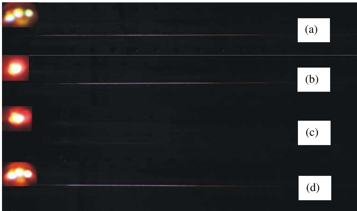
Fig. 14. Filament pattern at temperature of (a) 25 °C; (b) 200 °C; (c) 300 °C; (d) 25 °C. The inserted pattern in every picture is the output beam profile.
