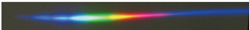
Fig. 14. Photo of the spectrally resolved filamentation output in the self-compression regime. Concerning the CEP stability of the filamentation output, several femtosecond filamentation experiments performed at various center wavelengths (Hauri et al., 2004, 2007) have clearly demonstrated that the filamentation process preserves the CEP stability of the input pulses. Therefore, we are convinced that the filamentation process does not degrade the CEP stability of the OPCPA input pulses in our experiment. Nevertheless, in order to quantify the quality of CEP stability, we are planning (i) to perform inline f -to- 2f interferometry to the OPCPA output of stages 3 and 4, (ii) quantify possible differential CEP drifts caused in the individual amplification stages 3 and 4 using a TADPOLE-type technique, (iii) and finally perform f -to- 3f interferometry (since a sizable third harmonic is generated inside the filament) to the filamentation output.
