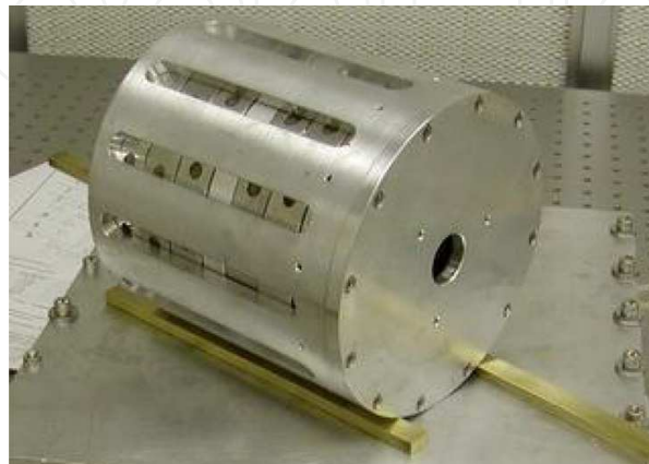
Faraday isolator for vacuum application
