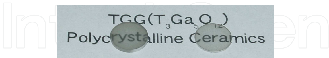
Fig. 4. A photograph of the first TGG ceramics samples made by A.Ikesue (Japan) in 2003.
