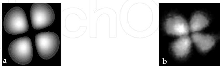
Fig. 3. Theoretical (a) and experimental (b) (Khazanov et al., 2000) intensity distributions of depolarized beam.
