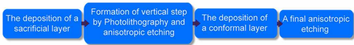
Fig. 1. Step Requirement for fabricating Nanowire using SPL
