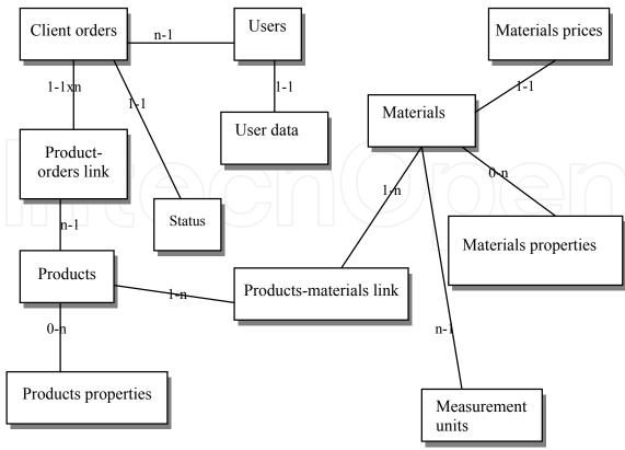
Fig. 11. Data base structure
