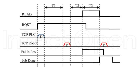
Fig. 13. Communication protocol between the PLC and a Robot Controller for authorizing an OH operation execution
