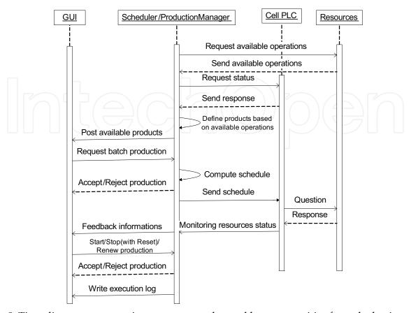
Fig. 8. Time diagram representing messages exchanged between entities from the business domain
