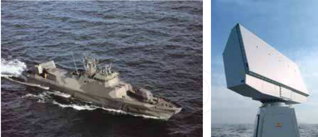
Fig. 21. TRS-3D on the Finnish guided missile boat "Hamina" (Photo courtesy of EADS)
