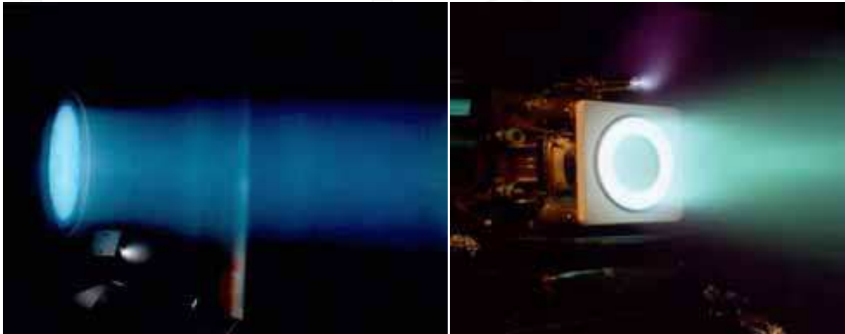
Fig. 4. The XIPS-25 firing (left) and the BPT-4000 thruster firing(right).
