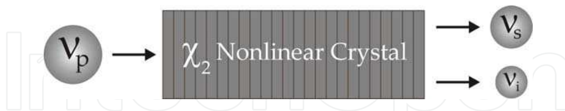
Fig. 1. The generation of long wavelength light through parametric frequency down-conversion. Here, v_p = v_s + v_i .
