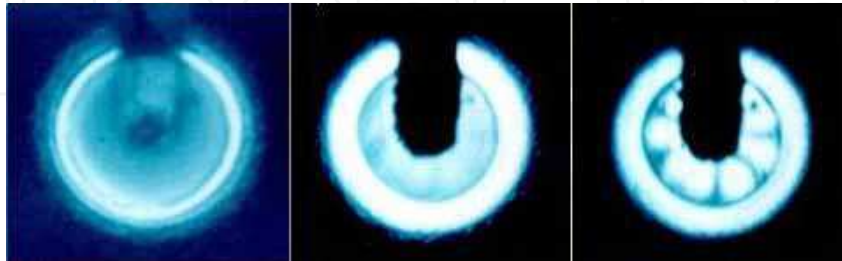
Fig. 2. CCD pictures of emissions at 12 \mu\text{A} , near PQR threshold, at 11.5 mA, below VCSEL threshold, and at 12.2 mA, above VCSEL threshold, respectively.
