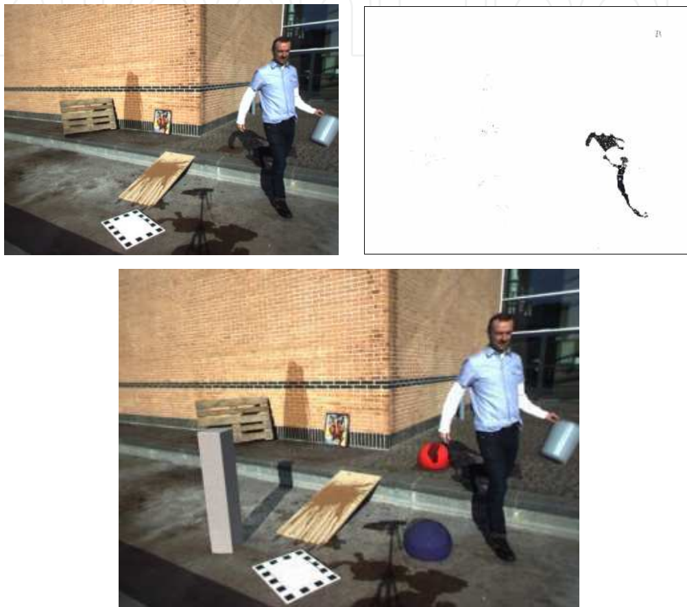
Fig. 3. Top left: input image containing walking person. Top right: detected dynamic shadow. Bottom: image augmented with virtual objects consistently shaded and casting shadows.
