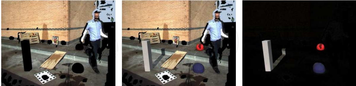
Fig. 9. Modelled part of scene rendered with no augmentation and masked with binary mask indicating augmented objects (left), is subtracted from scene rendered with augmented objects (center), yielding a difference image (right).
