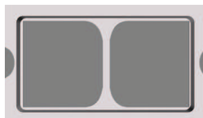
Fig. 3. Schematic of a silicon carbide tensile specimen in a silicon support frame
