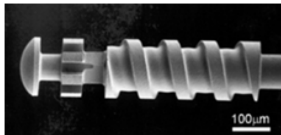
Fig. 3. A sample stainless-steel 3-D structure machined using a 5-axis \mu EDM system.
