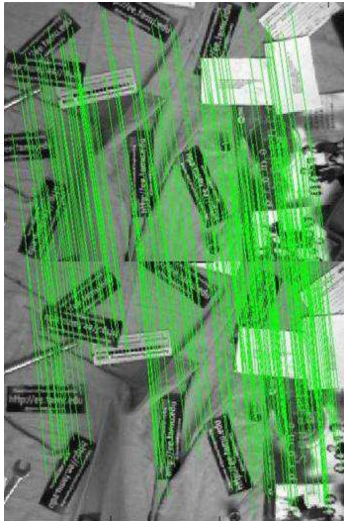
Fig. 5. Result of SIFT feature correspondence between two adjacent images obtained from a moving camera at different view points after data association.
