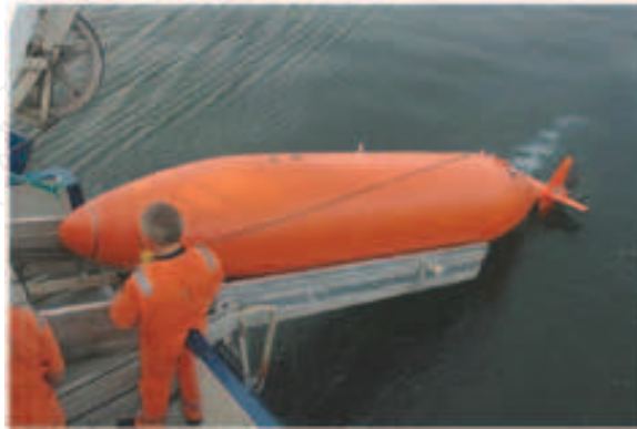
Fig. 1. The HUGIN 4500 autonomous underwater vehicle during deployment for sea trials (Kauske et al., 2007)
