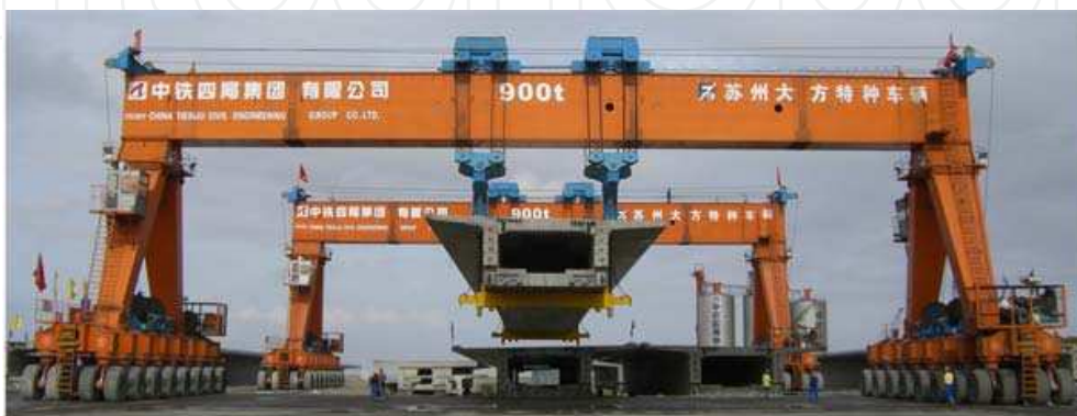
Fig. 1. Hoisting-girder transporter with 900T load
