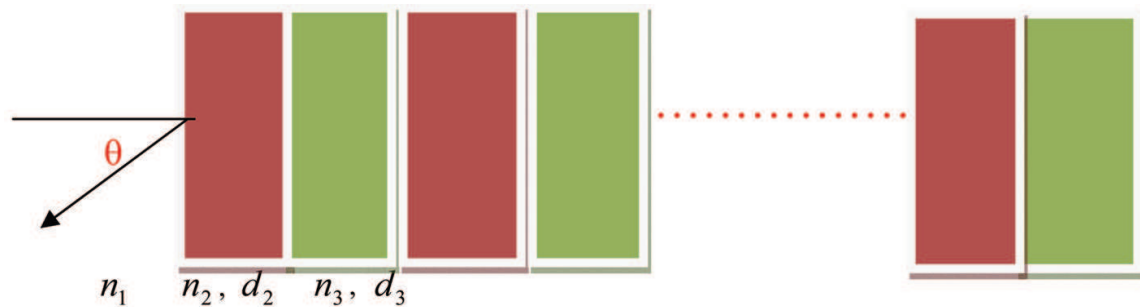
Fig. 1. Stack of 1 D MDPC ,where n_2 is the refractive index of the metal, d_2 is the thickness of the metal , n_3 is the refractive index of the dielectric material and d_3 is the thickness of the dielectric material.
