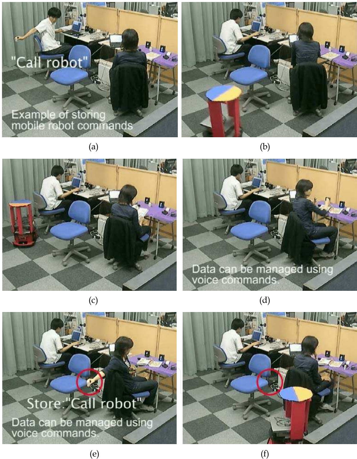
Fig. 4. Service execution using the spatial memory (a)request for "call robot" service by indicating the specified position, (b)(c)execution of "call robot" service, (d)service management by using a voice command, (e)storing the "call robot" service, (f)execution of "call robot" service
