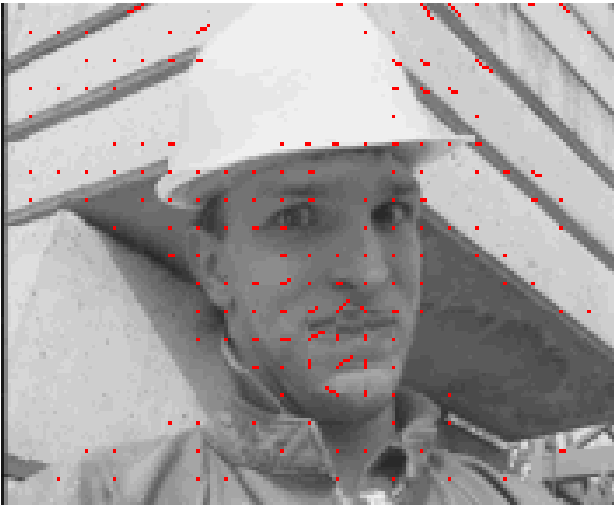
Fig. 20 (d). Motion field estimated by the Half Pixel RD with Embedded Algorithm scheme on the QCIF-Foreman sequence frame 204. The PSNR quality is 34.66 dB and it requires 889 bits to encode using the H.263 Huffman codebook.
