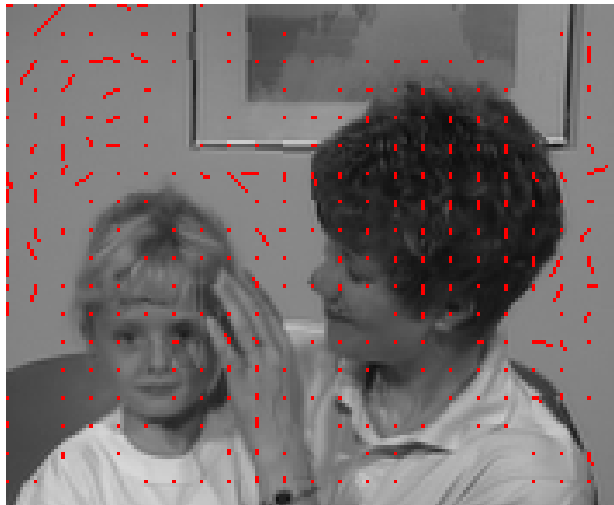
Fig. 21 (a). Motion field estimated by the conventional Half Pixel scheme on the QCIF-Mother & Daughter sequence frame 28. The PSNR quality is 34.83 dB and it requires 1476 bits to encode using the H.263 Huffman codebook.
