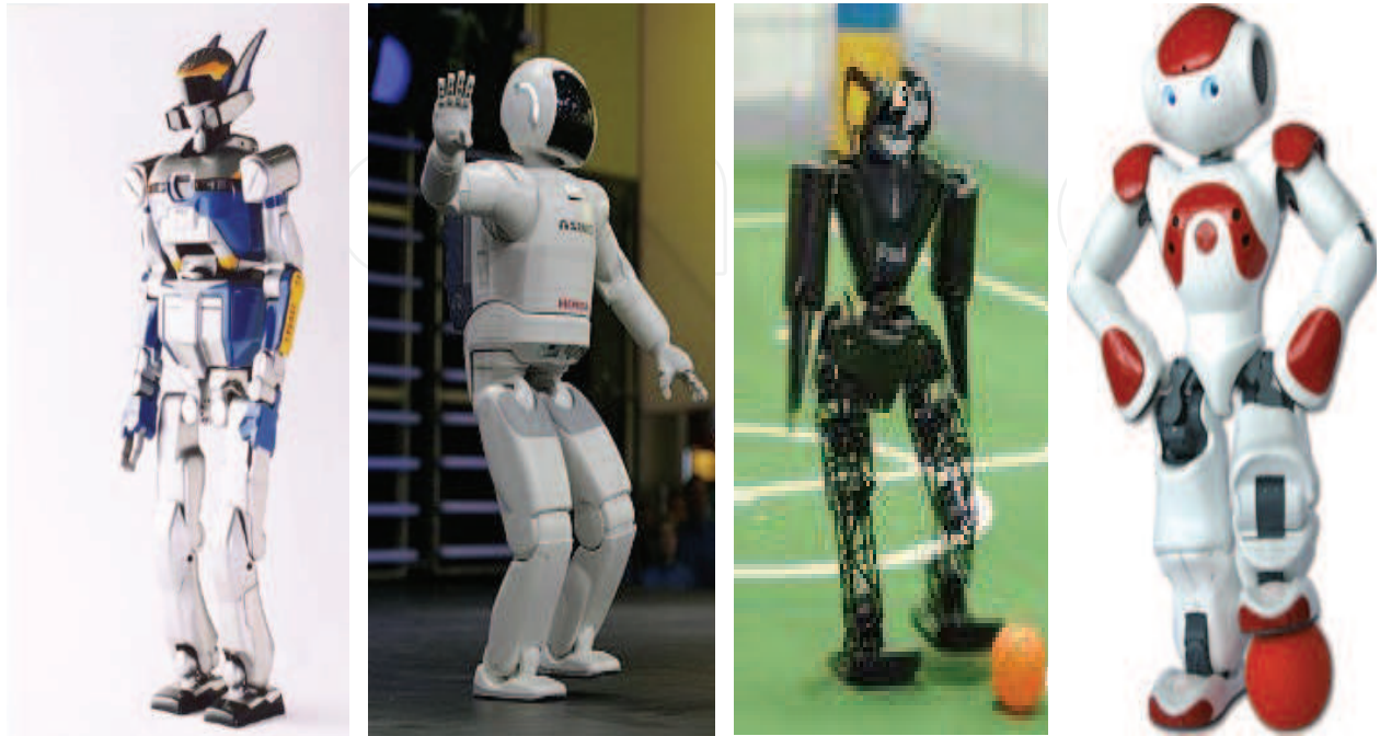
(a) 2 (b) 3 (c) 4 (d) 5 Fig. 1. Humanoid robots: (a) and (b) are human size robots, (c) and (d) are middle size robots. (a) HRP2, (b) ASSIMO, (c) Nimbro soccer robot, (d) NAO robot.
