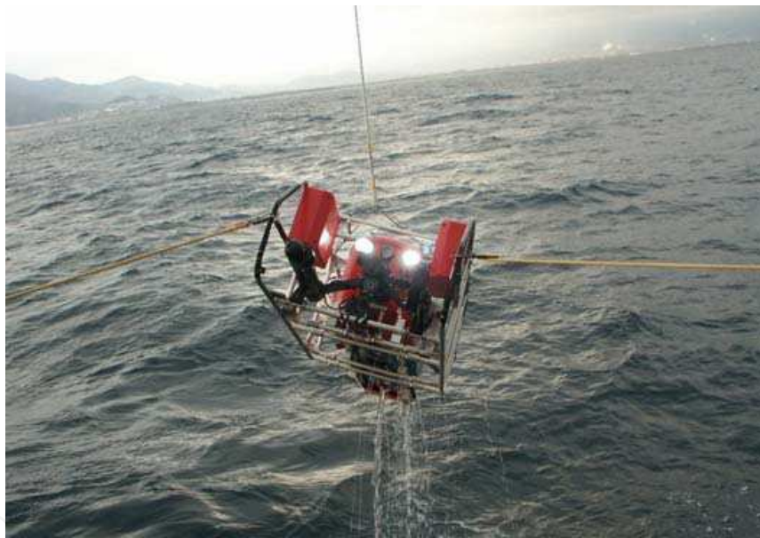
Fig. 14. PICASSO-1 with the Visual Plankton Recorder being recovered.
