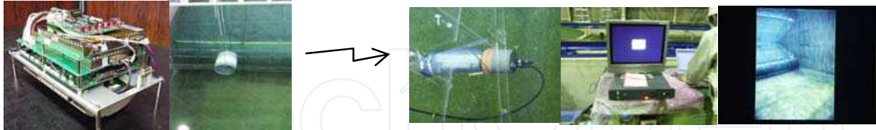
Fig. 8. Picture of ELF wave transceiver tested in tap water and a received image.
