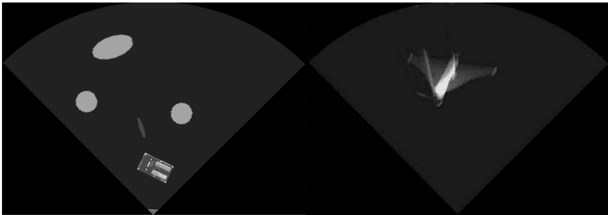
Fig. 8. The resulting images of the simulated Forward look sonar.
