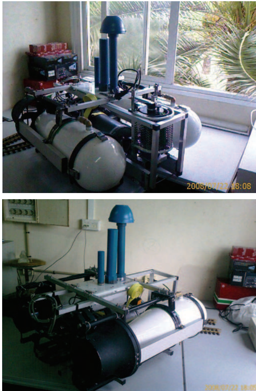
Fig. 4. Photographs of the low-cost ICTIOBOT prototype system, the EN4AUV introduced earlier. It has been developed using CLIPS that constitutes a C language based shell, and allows the knowledge representation to be in the form of rules and frames (COOL or Clips Object Oriented Language). These formalisms are used in the knowledge base (KB) to represent the involved knowledge. The main feature of the expert system is to assess a current situation in order to act accordingly, in a clearly data driven/reactive behavior. Thus, EN4AUV is a reactive expert system, taking the proper action for every different situation, and considering the pipeline/cable status, the type of survey, the different mission settings, and others.
