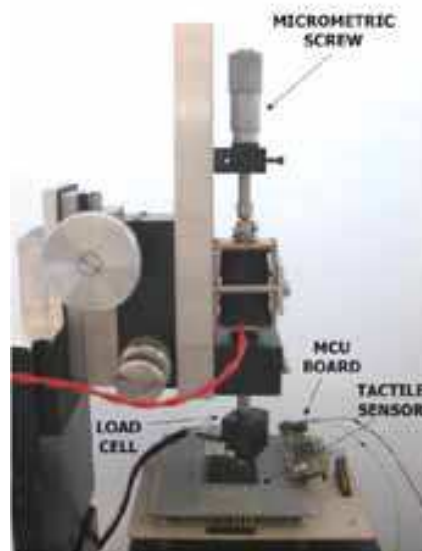
Fig. 22. Test rig for sensor calibration and tests.
