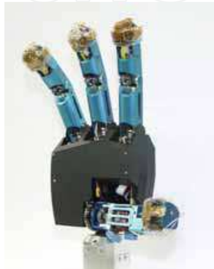
Fig. 1. SKKU Hand II with tactile sensor
