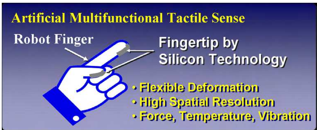
Fig. 1. A future image of tactile imager embedded in robot fingers. They will function as artificial tactile sense of fingertips in human-coexistence type robots.
